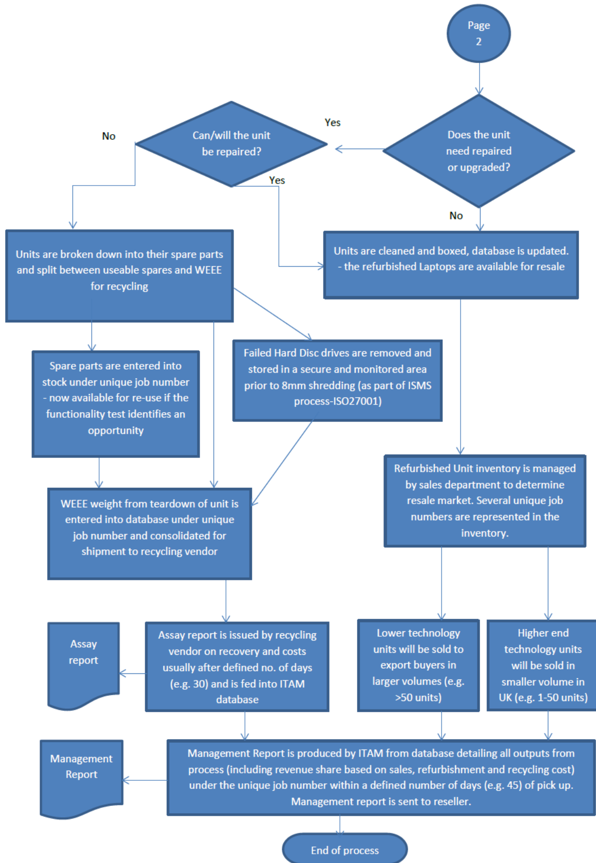
Figure 4 (Cont/...). Laptop Refurbishment/Resale Flow Diagram
